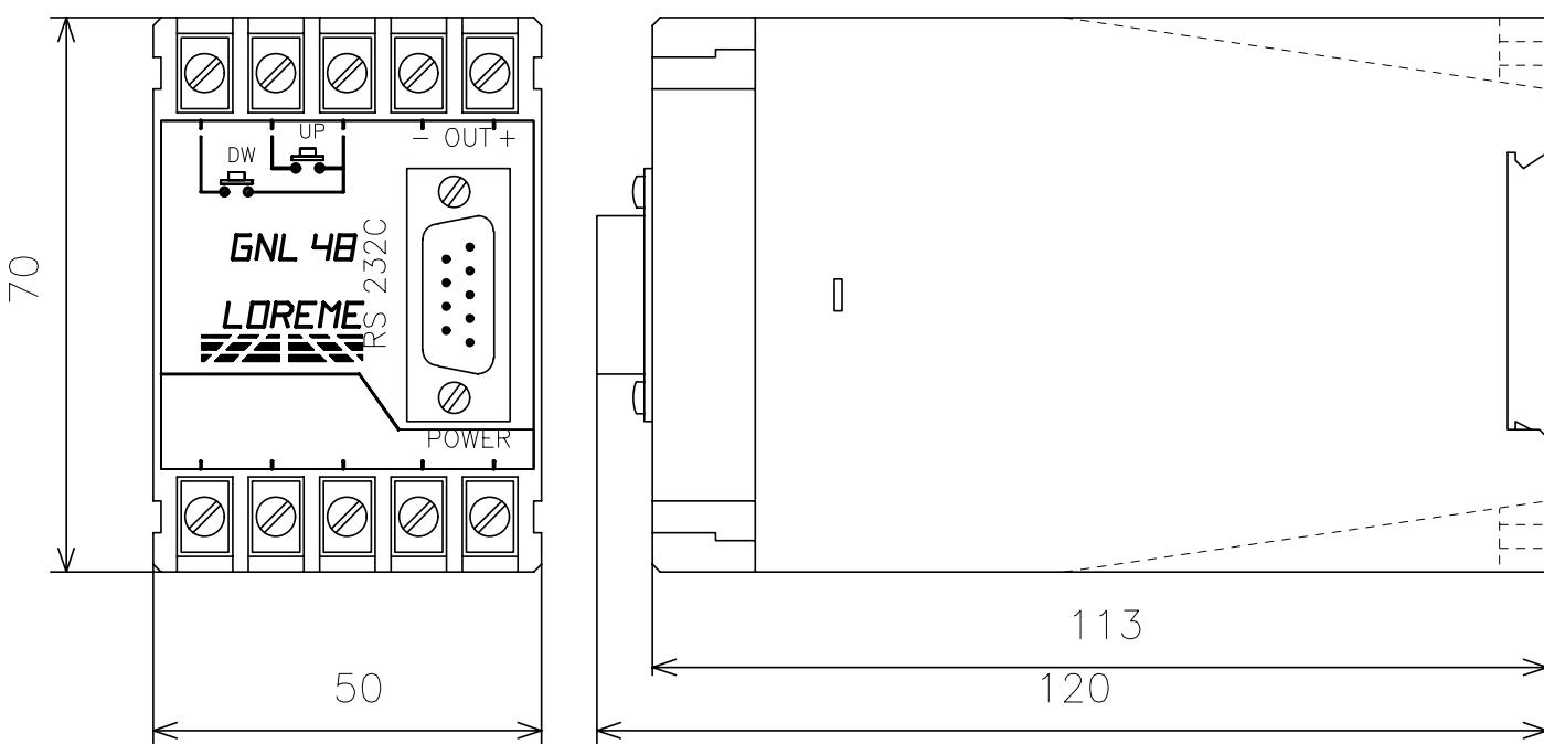
To guarantee their technical specifications we recommend a spacing of at least 5 mm between each apparatus
